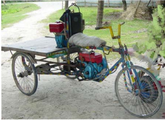
Figure One: Motorized rickshaw flatbed with 3.5 HP mover with 3 HP Chinese engine near Tongail bazaar
